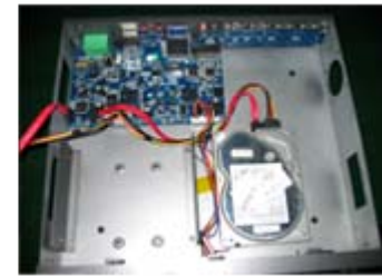
⑥ connect the power wire and Cable
